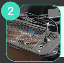
Make sure that your Linkbox (Usb and Displayport) is connected to the computer and to an electrical socket
