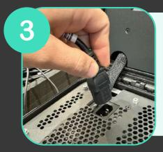
Connect the power supply to an electrical socket
