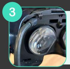
Make sure your headset is plugged into the Linkbox and switch it on
