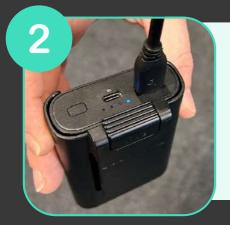
Connect your Vive Wireless adapter to the Powerbank using the USB cable
